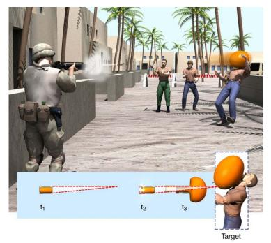
Application of the LPS (OPS) with variable-range kinetic energy munition with inflating bag.
