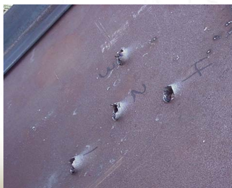
Back Side of 2" Armor Plate (3km equivalent)
