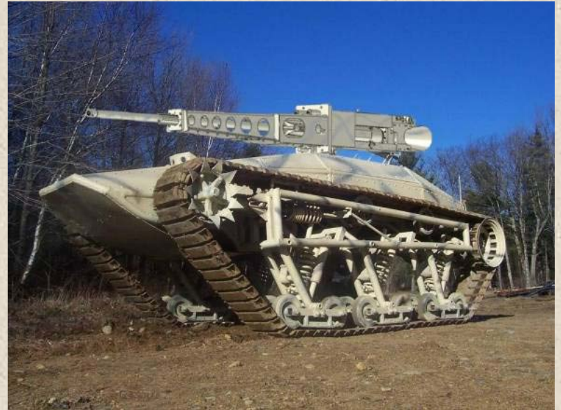
Notional 45mm RAVEN Automatic Cannon Mounted upon a RIPSAN Robotic Vehicle
