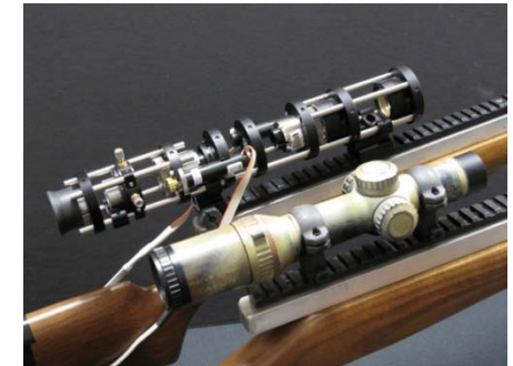
Figure 0. Barrel position sensor and reticle compensation system.
