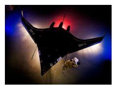
(scaled-down wind-tunnel model) BWB quiet aircraft: range & payload  $\times$ ~2, sorties  $\div$  5–10, fuel  $\div$  5–9 ( $\Sigma$  2–4)
