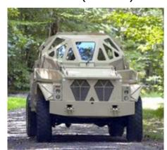
More lethal, highly IED-resistant, stable HMMVV replacement, weight ÷ 3, fuel ÷ >3 (up-armored HMMVV ~4 mpg)
