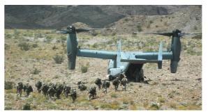
Optimum Speed Tilt Rotor (OSTR): range × 5–6, speed × 3, quiet, fuel ÷ 5–6
