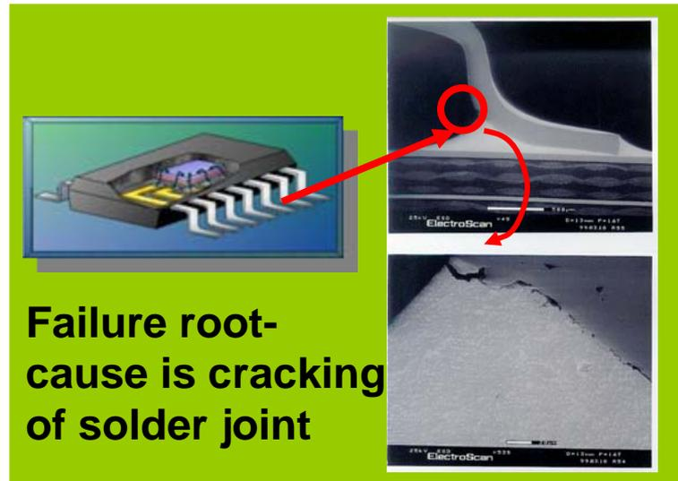
Failure root-cause is cracking of solder joint
