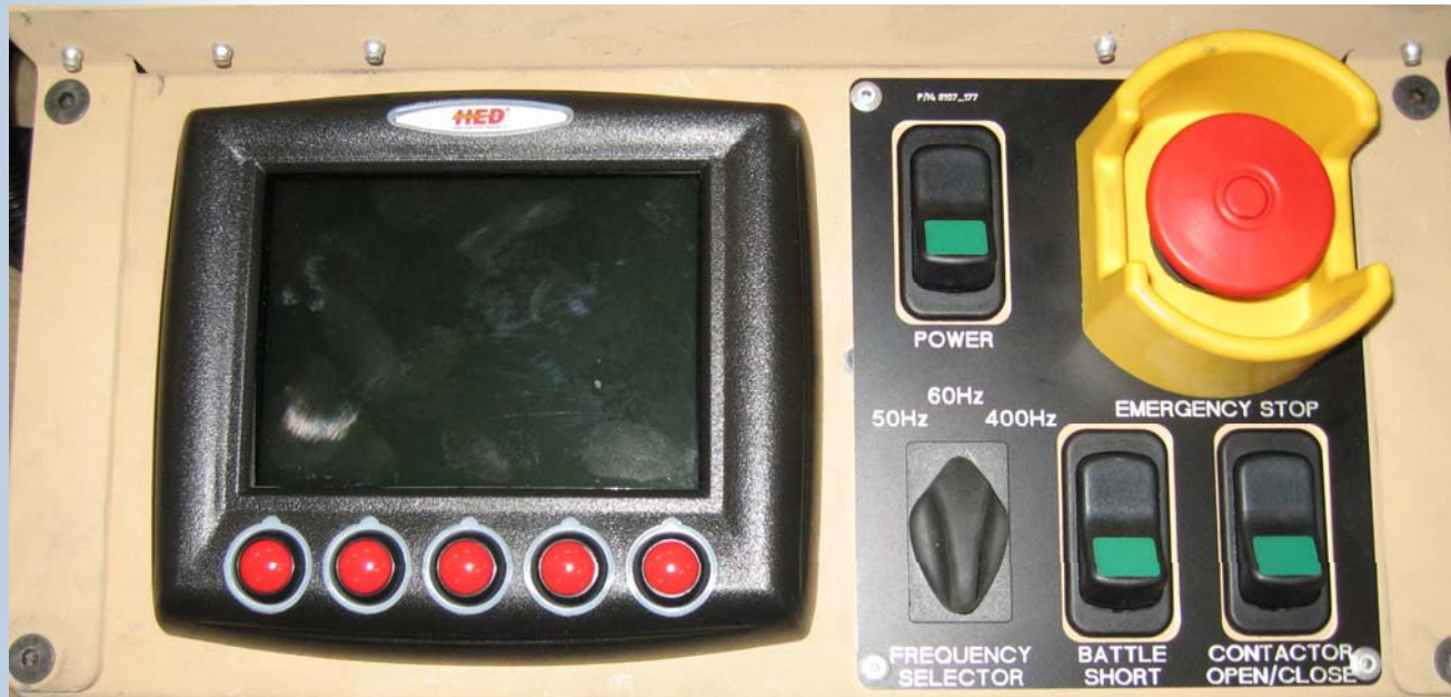
Operator Interface Panel
