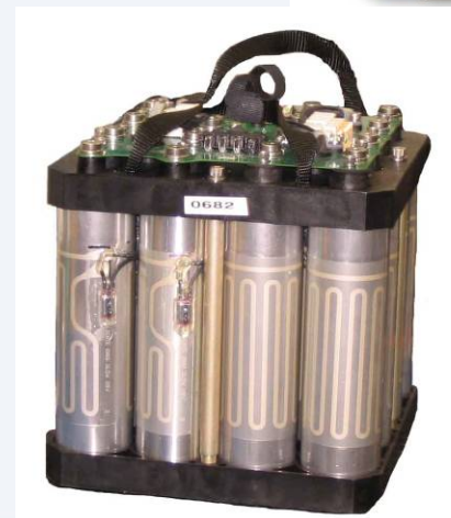
ITAS cell pack: 8S, 2P configuration
