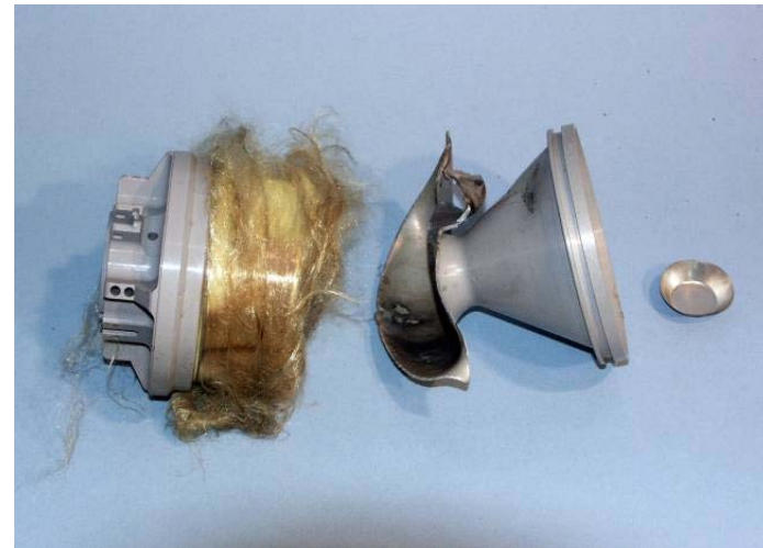
Remaining parts of Launch motor after FCO test with LPG.
