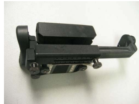
Test rig redesigned to accommodate lateral positioning 2cm closer to the face for offset sights
