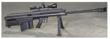
XM500 AMR .50 Caliber 26 lbs (Gas Op. Semi) – Lighter / Shorter than M107 at 46 inches long
