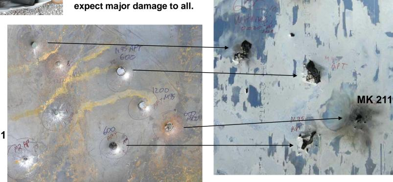
1/4 inch A36 Steel1/4 inch mild steel "Behind Target Effects" are more significant for@ 600 yards1/4 inch mild steel "Behind Target Effects" are more significant forM95 APT 20mm than for exploding MK 211 rounds at 600 yards.
