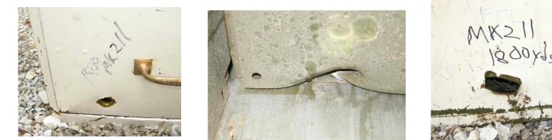
1800 yard MK 211 into target face and completely penetrated without activation
