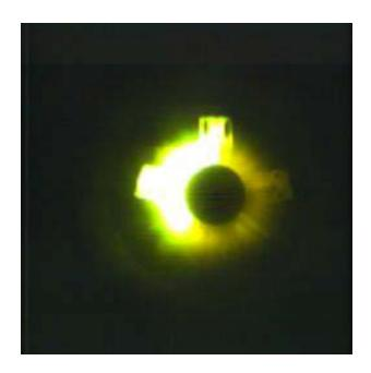
The small amount of light indicates that the round is just beginning to exit the gun. A short time later, more light at the left of the gun indicates asymmetrical gas leakage, which may adversely affect the flight.
