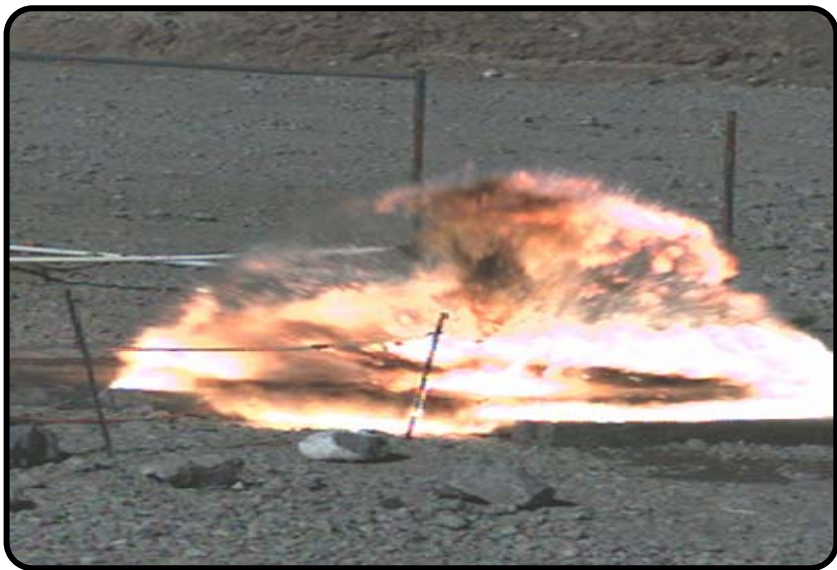
HME explosive performance evaluation test
