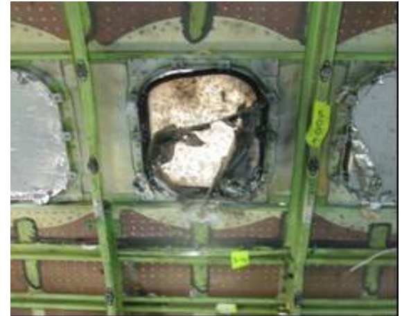
BPW Liner, Post-test (Interior View)
