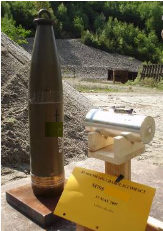
Test Set-up with 81mm SCJ
