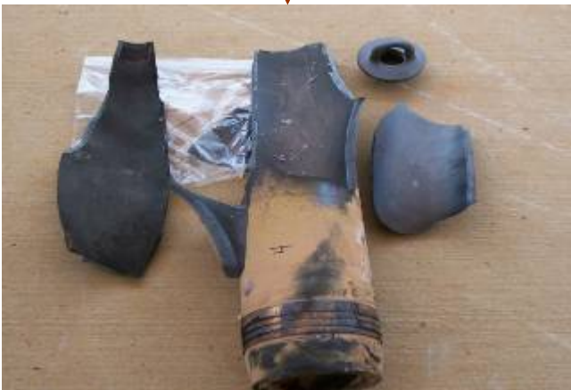
Without adequate venting
