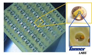
Micro-scale initiators on a PCboard substrate
