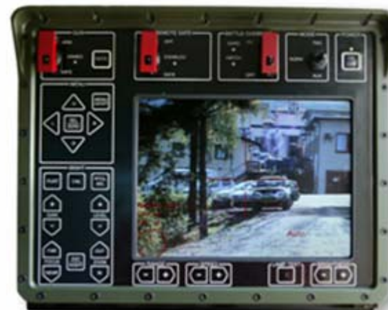
Fire Control Unit (FCU)
