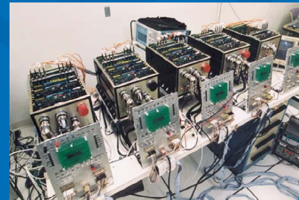
X-38 Fault Tolerant Parallel Processor 2-Fault Tolerant Flight Computer
