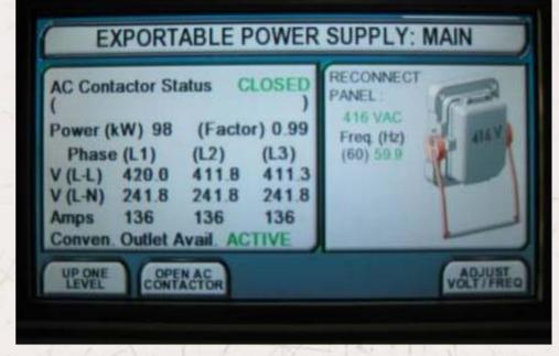
AC contactor on/off (turning on and off output power)
