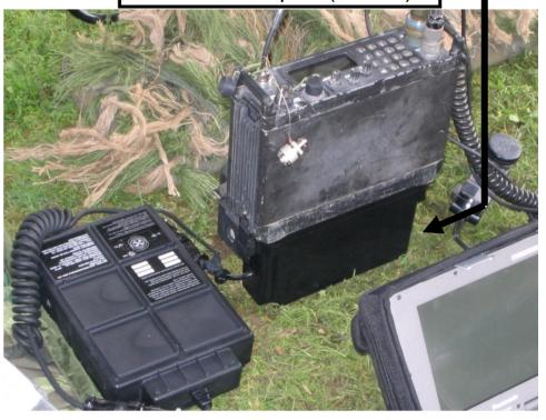
The BA-5390 has not been approved for use in any 24V radio system (refer to TAB B).
