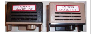
PP-8497/U Self-Discharge Device (CAP), black, tan or dual colored, is used to discharge (condition) the BB-390B/U or "Quick Check" that both 12-volt sections of the battery are working. When used with the BB-2590/U, it is only used to provide a "Quick Check". The BB-2590/U does not require conditioning.
