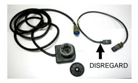
J-6362A/U DC slave cable for the PP-8498A/U (SPC). Disregard the smaller cable (attached), it is only used with the legacy PP-8444A/U.
