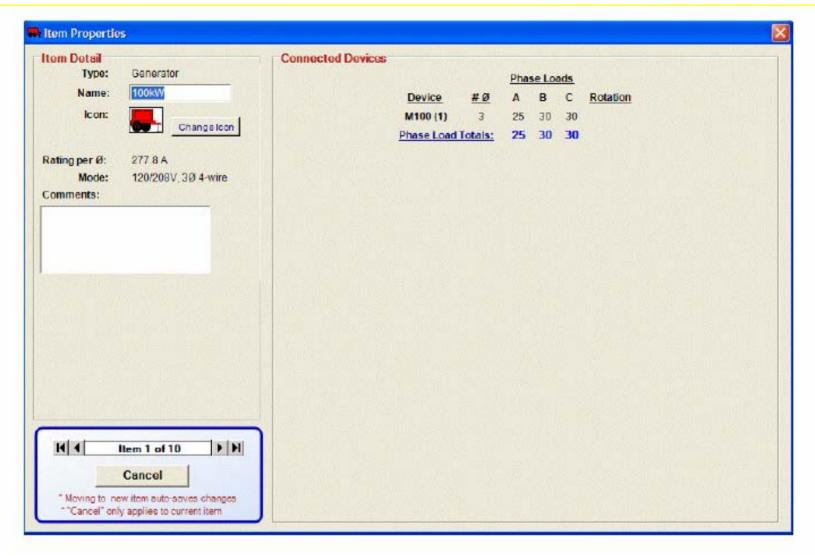
Ability to view each generator set and connected devices with load and phase details.
