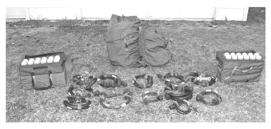
Used for Tent lighting and general electrical hook-ups 12 different wire assemblies + light bulbs
