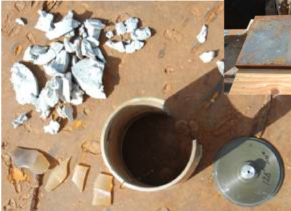
Typical type 4 reaction showing large chunks of unreacted explosive
