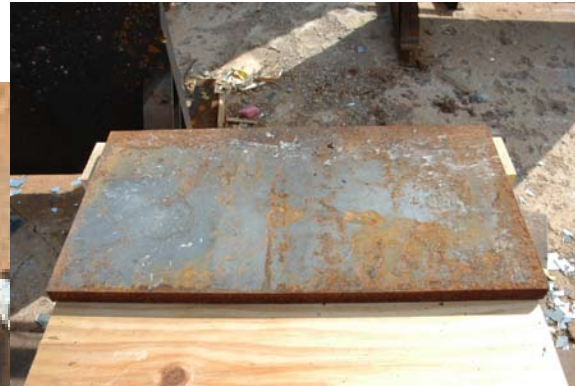
Witness plate after type 4 reaction
