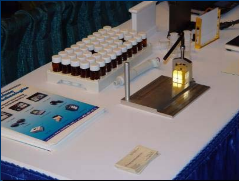
Propellant crusher, vial rack, dip basket with plate
