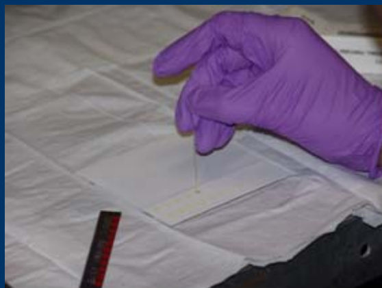
2) Dissolved propellants are spotted onto TLC plate
