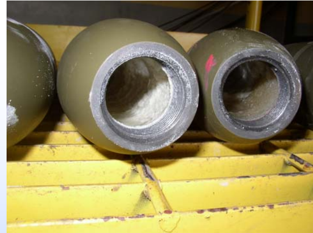
Shells after one 30 second cycle of cleaning.
