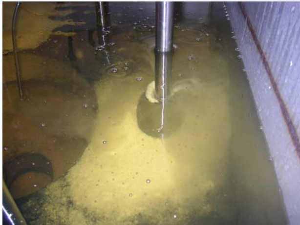
Probes sonicating inert material in shells.
