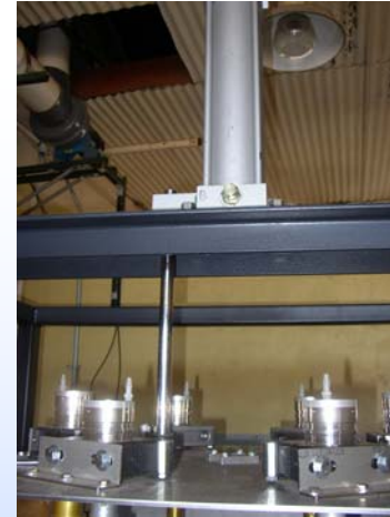
Lift plate holds 6 sonic probe converters.
