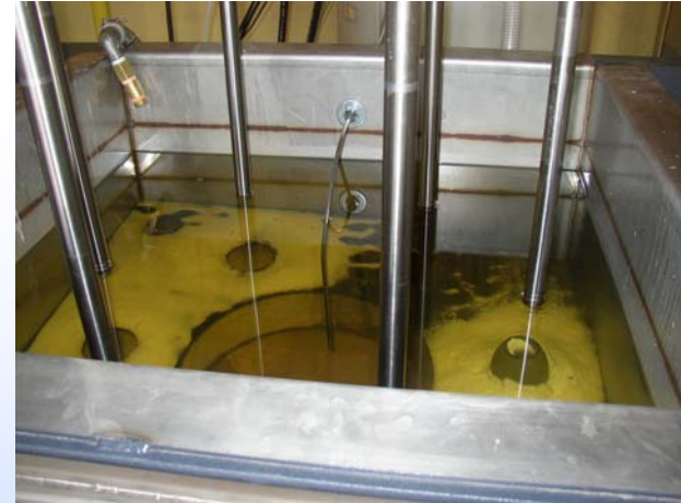
Sonication tank with removed inert material .
