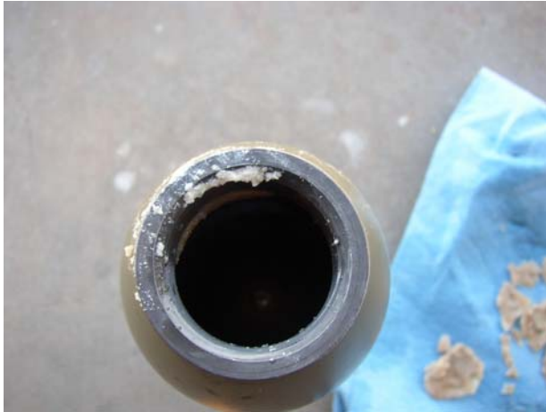
81mm shell with inert material removed.
