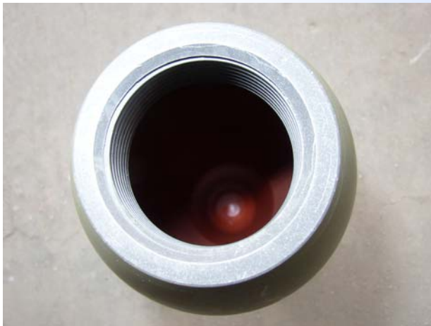
Shell after two 30 second cycles of cleaning. All inert material was removed.
