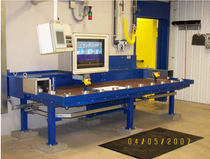
Input Conveyor and Control Station for Disassembly Machine
