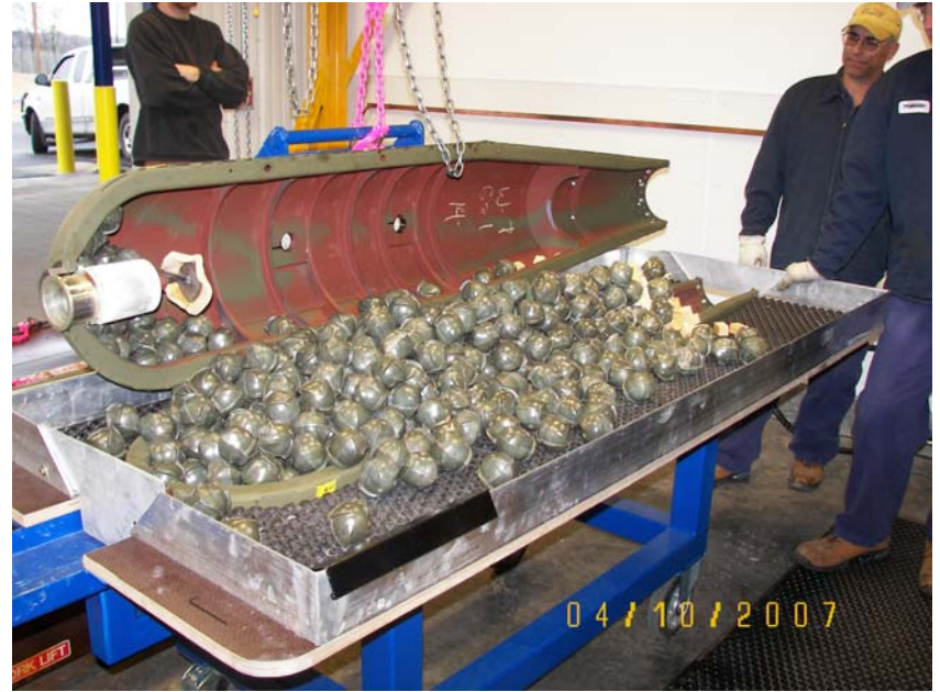
Fixture for Opening CBU Dispenser
