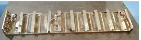
6"X30" & Full 75" Sidewall Fuel-Cooled Heat Exchanger Demonstrated Structural Durability
