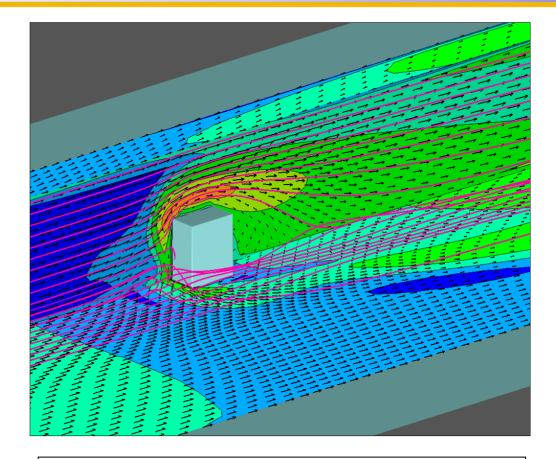
Streamlines and wind vectors from RUSTIC simulation of flow around a cube in a channel. Contours are of TKE.
