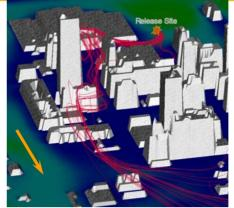
Streamlines Predicted by RUSTIC in OK City. Turbulence<sup>®</sup> Produces Complex and Nonintuitive Flow (above).
