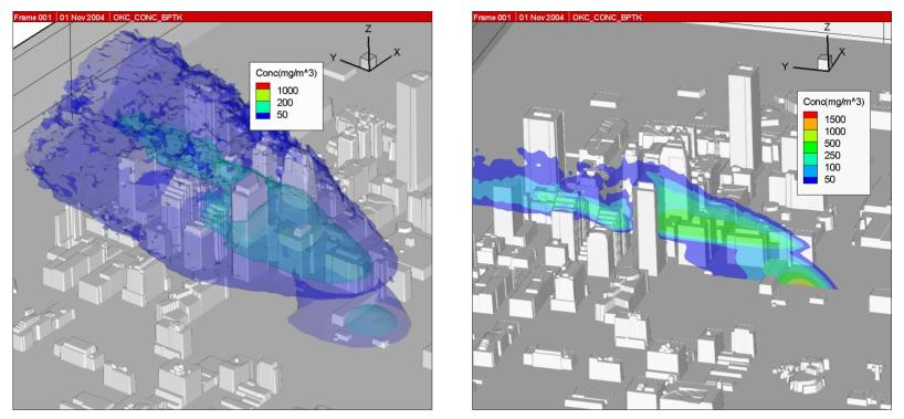
Simulated concentration levels for volatile drops release in Oklahoma City
