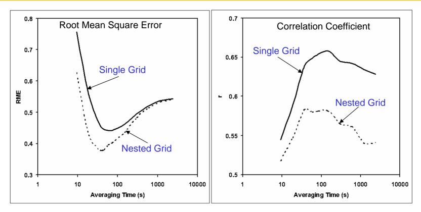
•Little change in correlation between model and sonic anemometers for averaging times from 40 seconds to 2400 seconds.
