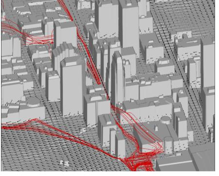
2. Use MESO to compute contaminant dispersion with flow and turbulence predicted by RUSTIC.
