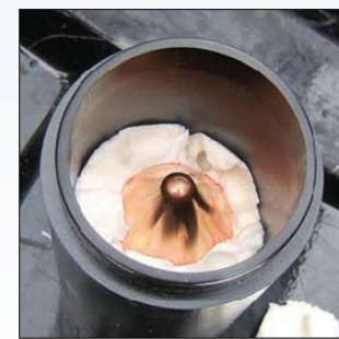
Shaped Charge Assembly for Remote Destruction of Buried IEDs
