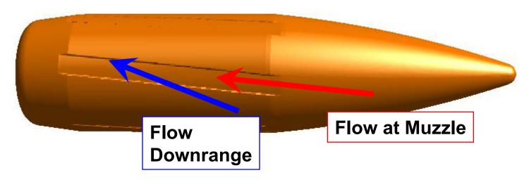
• An important focus: effect of engraving on aerodynamics
