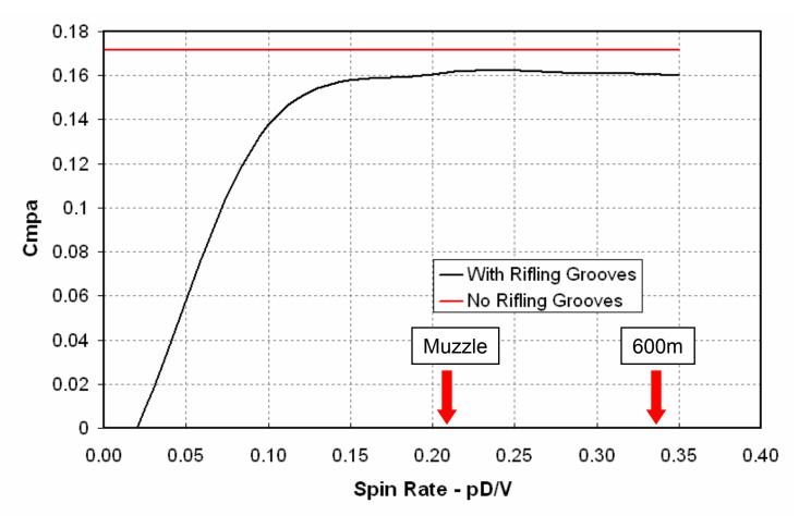
For 5.56mm ammo, slight offset in side moment affects Magnus moment only at low spin rates. Demonstrates that special twist rate guns (match spin) <u>not</u> required for aeroballistic testing!
