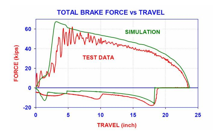
ATD #1 RECOIL SYSTEM TEST RESPONSETEST ROUND #3 (7/20/04) M829A2 w/ 10 ROWS MUZZLE BRAKE HOLES
