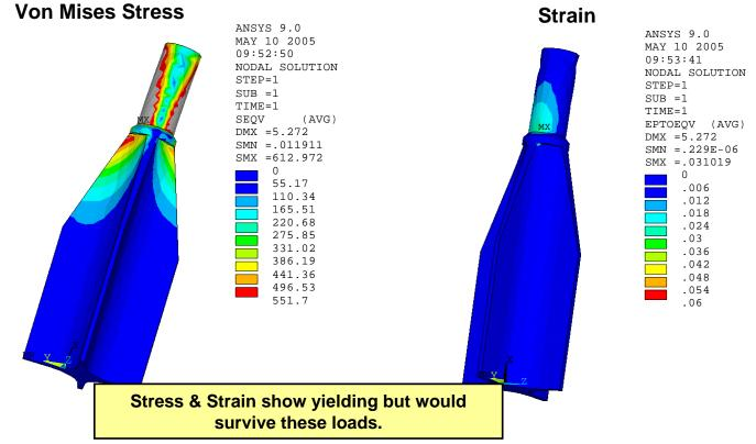
Red Lion EM ILP Test120 Fin Alum 30kg's axial, 11kg's trans May 10 05 Test120 Fin Alum 30kg's axial, 11kg's trans May 10 05
