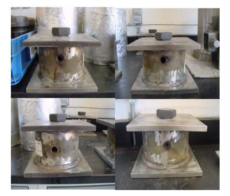
*I-TNT demonstrated No Reaction in four Bullet Impact tests using 4" long 155mm case sections.*
