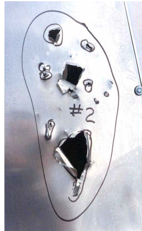
SPALL AND FRAGMENT SIGNATURE ON WITNESS PANEL
