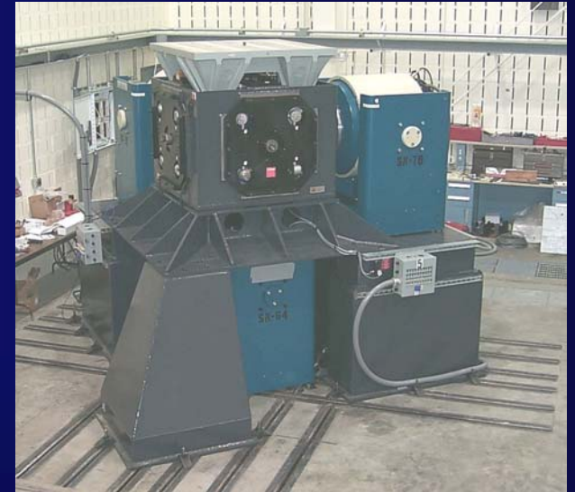
NAVSEA Keyport's 3-Axis Electrodynamic Vibration Test System
