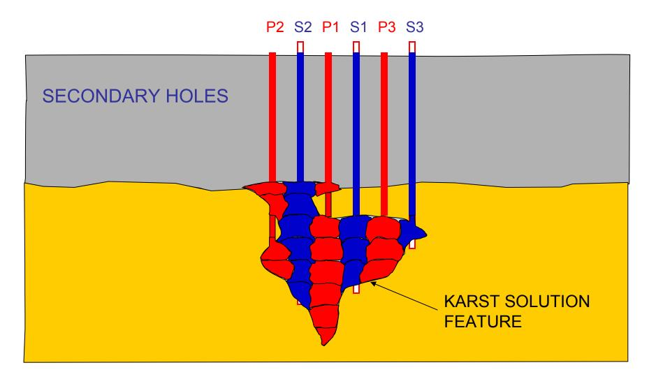
Solution Feature Remediation (Upstage Casing Extraction (LMG or HMG)
