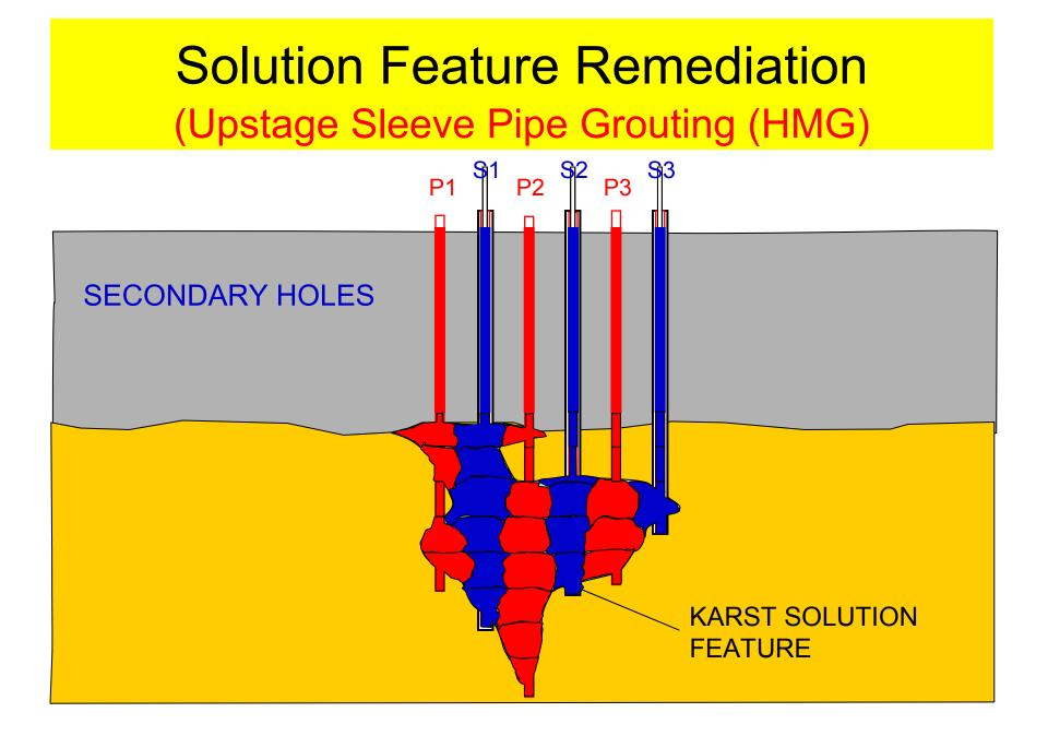
Solution Feature Remediation (Upstage Sleeve Pipe Grouting (HMG)
