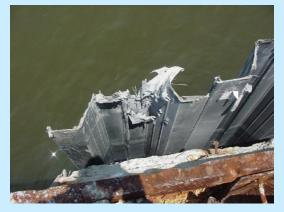
for use. In the meantime, vinyl sheet piling should not be used in applications where life safety and widespread property damage are at stake in the event of failure.
