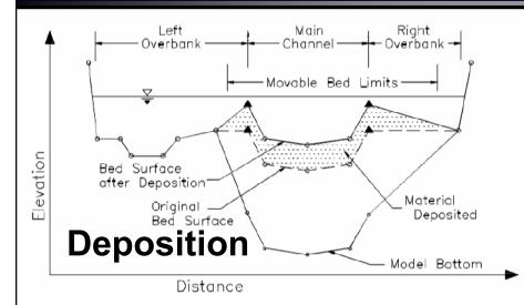
RAS computations modified to compute bed changes and modify cross sections before each time step
