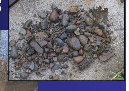
Sediment accumulated in Station 45+00 weir box
