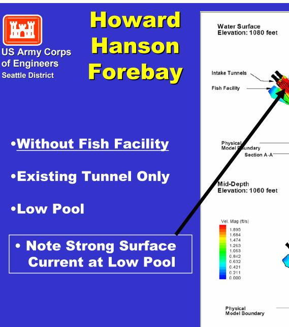
Appendix Figure 5: Plan View of Velocity Magnitude at Water Surface and Mid-Depth
