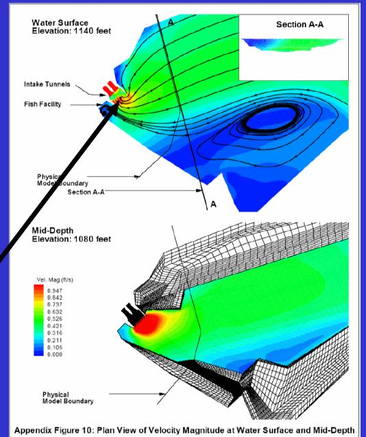
Scenario S5P2: Tunnel: 4000 cfs. Fish: 0 cfs
