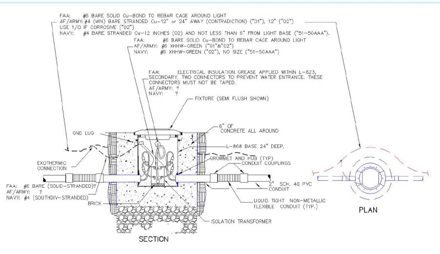
L-868 BASE DEEP CAN METHOD (GREEN GROUNDING CONDUCTOR CONNECTED TO COUNTERPOISE)
