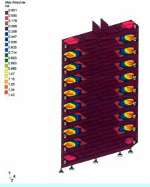
**Figure-6 Stress Contour (Wheel load)**
