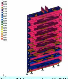
Figure-2 Stress contour (Self Weight)
