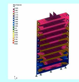
Figure-5 Stress Contour (Down pull load)
