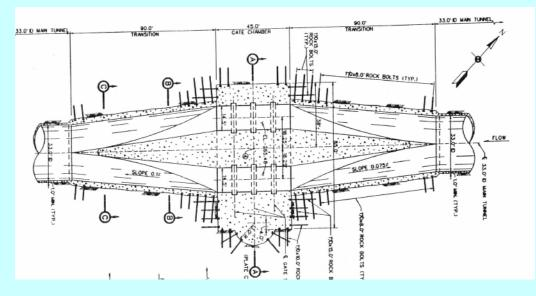
PLAN VIEW OF THE WHEEL GATES (MAIN TUNNEL)
