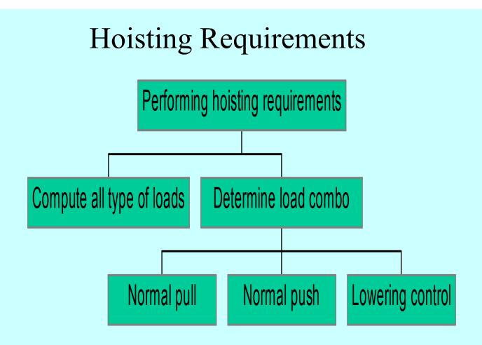
**NOTE:** Hoisting requirements are determined to estimate cylinder size and max. push requirements.
