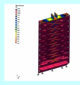
Figure-7 Stress Contour (Machinery load)
