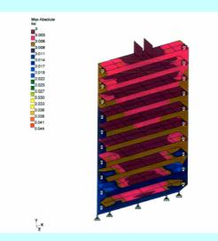
Figure-8 Stress Contour (Bouyancy load)
