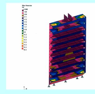
Figure-3 Stress contour (Hydrostatic load)
