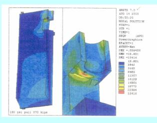
Figure-4: Gate slot cut-out close-up view (ANSYS)
