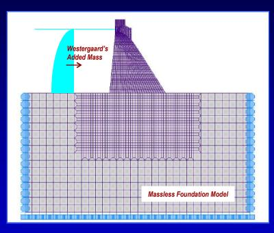
Finite-element mesh for spillway Monolith 14
