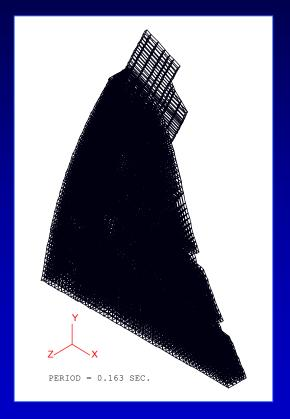
Fundamental mode shape  $T_1 = 0.163 \text{ sec} (f_1 = 6.14 \text{ Hz})$
