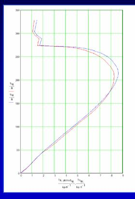
Inertia forces associated with fundamental mode response
