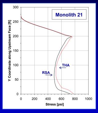
$RSA \rightarrow Maximum stress estimate$ obtained with the response spectrum approach considering horizontal and vertical input ground motion.
