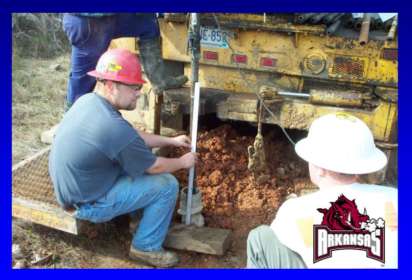
Instrumented Drill Rod to Measure Hammer Energy
