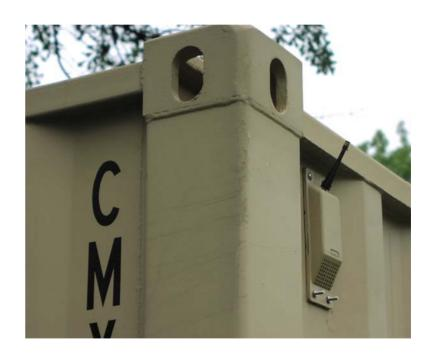
USMC TRICON with prototype Integrated Sensor / RFID
