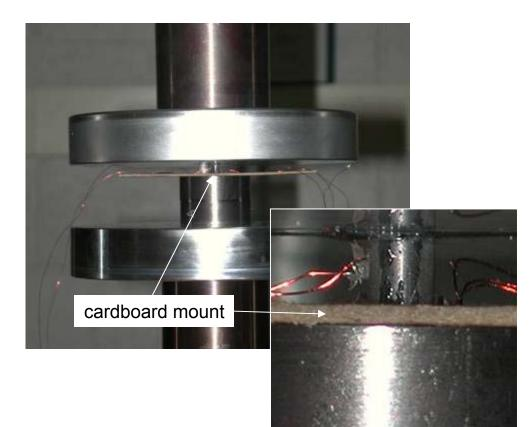
One axial strain gage and one rosette gage were set 180° apart. Cardboard mount were used to ease the handling of the specimen during experiment.
