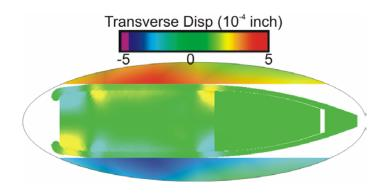
Transverse Displacement of the Projectile at Peak Acceleration
