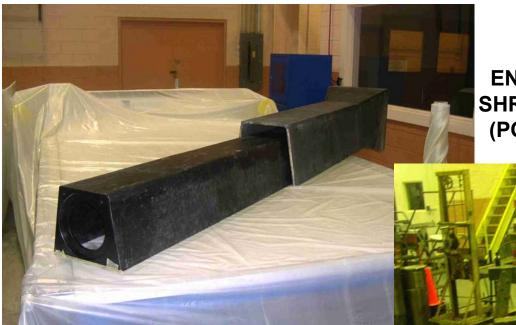
ENVIRONMENTAL/SIGNATURE SHROUD COMPOSITE SECTIONS (POST CURE) MADE AT BENET
