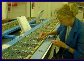
**Thru-Hole PWB Assembly**
