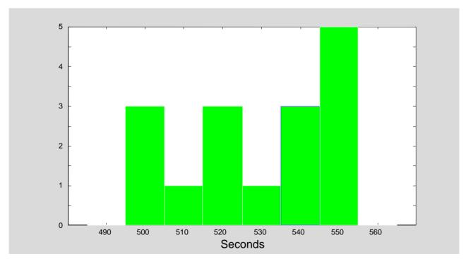
Power supply life is a conservative measure of fuze operational life. (1 Megohm loading of 3.3 volt buss) Test conditions: FFCS pulse = 195 V, 15 ms Temperature = 68°F
