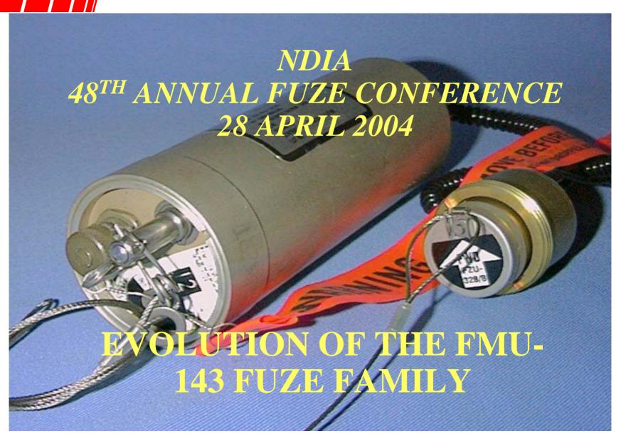
The FMU-143B/B fuze was developed for the **U.S. Air Force for Hard Target Penetration** when used with the BLU-109 and Precision Guided Munitions (PGM) systems. Over the last eight years, the FMU-143 has been modified to meet customer requirements for several different systems. This presentation will cover variations and approach as the family evolved.
